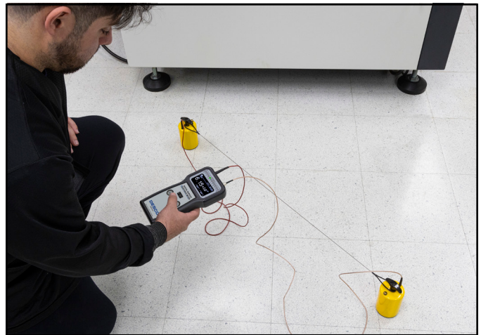
Figure 14. Measuring the Resistance Point-to-Point (R tt ) of floor materials
